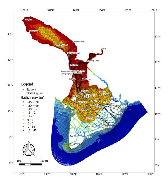
Figure 7. River bathymetry from cross-section interpolation and shelf bathymetry of the Mekong Delta.
