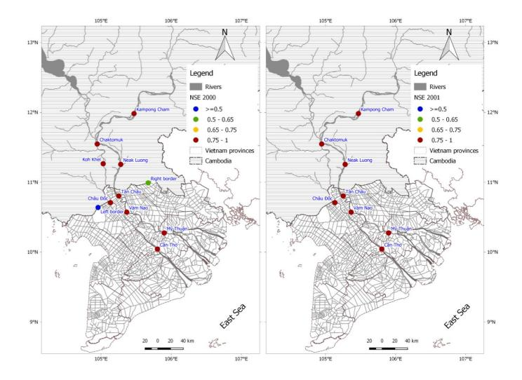
Figure 9. NSE values of water discharges at the gauging stations in the Mekong Delta. The calibration (the year 2000) and validation (the year 2001) are presented on the left and right maps respectively.
