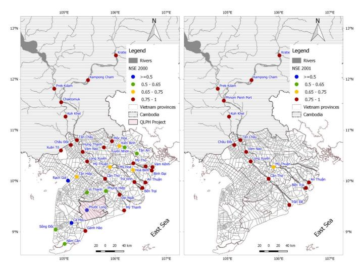
Figure 8. NSE values of water levels at the gauging stations in the Mekong Delta. The calibration (the year 2000) and validation (the year 2001) are presented on the left and right maps respectively.
